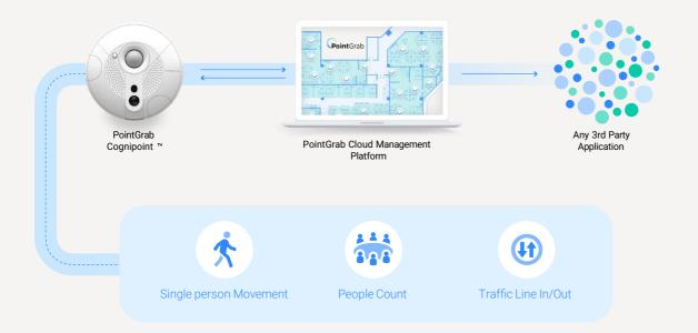
As a market leading technology, the PointGrab Sensing Data System is capable to provide real-time and historical drill down insights into the actual behavior of sites, building, floor, rooms and even a single desk or equipment.
